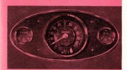
Centrally placed on the dash, the instrument panel contains three easy-to-read instruments. The speedometer contains a fuel gauge, while separate gauges are provided for water temperatures and oil pressure.
