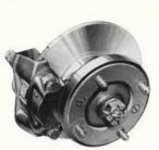
A fast car must be able to stop — fast! 7 in. front disc brakes provide the necessary confidence for high-speed travel.
