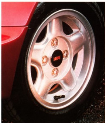
Giving an edge to that legendary handling, the Cabriolet is fitted with 5-spoke Revolution alloy wheels with 165/60 X 12 low profile tyres.
