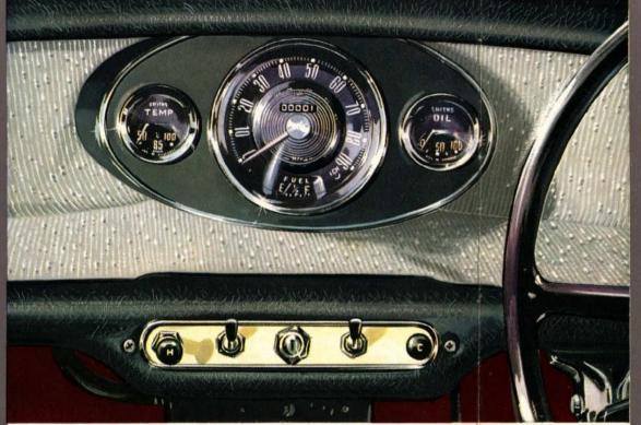
The fascia panel contains a comprehensive selection of instruments grouped in a symmetrical three-dial arrangement. The large speedometer and mileage recorder contains a fuel gauge. The two smaller dials show water temperature and engine oil pressure. Positive-action toggle switches control the lights, and a key switch opens or closes the ignition circuit and operates the starter solenoid switch.
