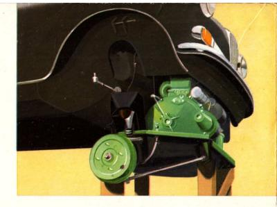
Within an overall car length of only 10 ft. 83 in. (3.270 m.) there is more passenger and luggage room than is usually acceptable in a 1½-litre saloon. The entire engine/transmission unit, together with the front suspension and steering gear, is contained in one compact assembly. Aft of this there are no mechanical encumbrances to intrude upon passenger space.
